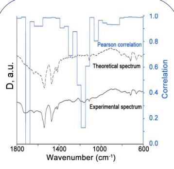
Pearson correlation analysis of FTIR spectra for binary mixtures of BLPE and magnesium stearate
