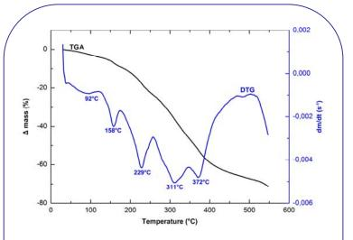
TGA-DTG profiles of bilberry leaf powder extract with the indication of peak temperatures of mass loss events
